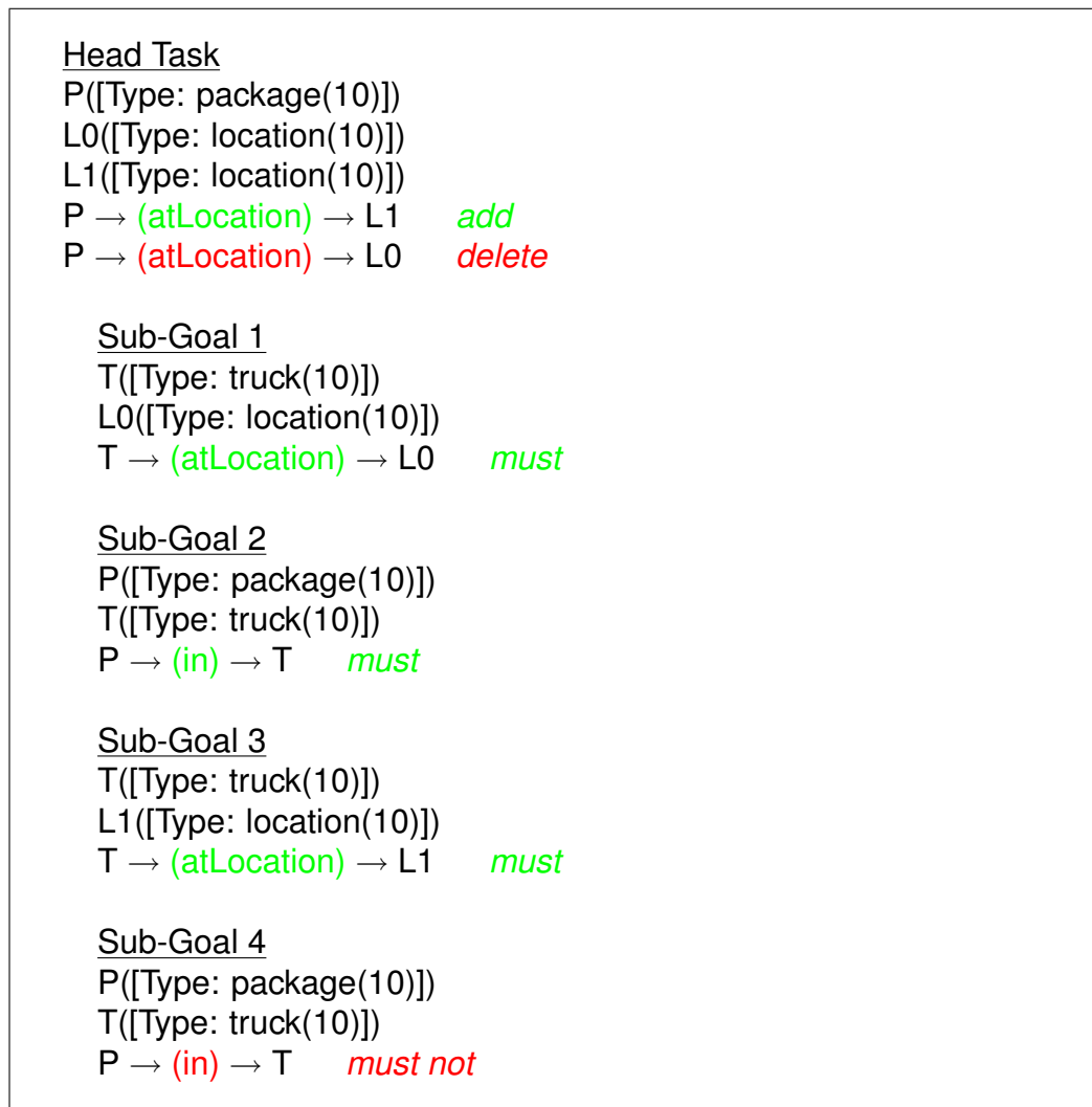
Figure 4.9: Decomposition rule for delivering a package
